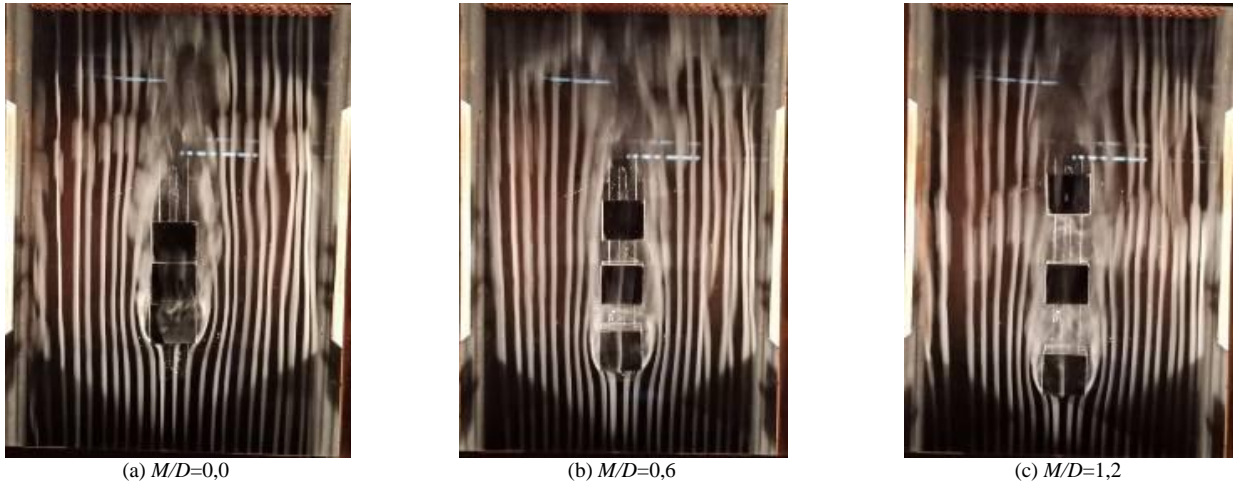
Figs. 7. Visualization of flow in three tandem square cylinder in model II serial configurations or (a) M/D and N/D=0.0 ; (b) M/D and N/D=0.6 and (c) M/D and N/D=1.2 at Re=43,844
