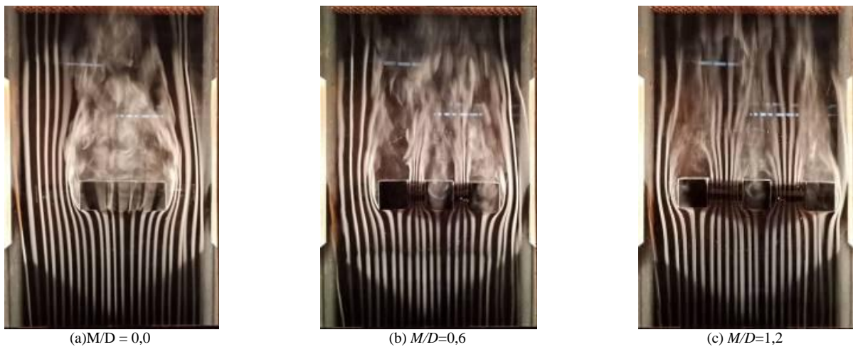
Figs. 8. Visualization of flow in three tandem square cylinder in parallel configuration model I or (a) M/D=0.0 ; (b) M/D=0.6 and (c) M/D=1.2 while N/D is constant at 1.2 at Re=43,844
